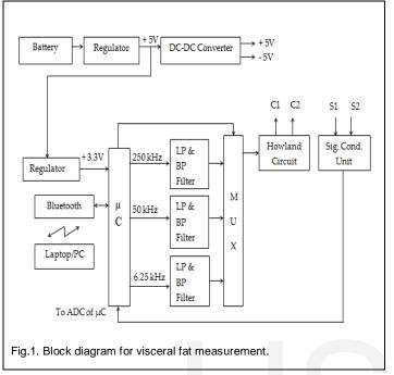
signal developed along the current path is sensed with the help of sensing electrodes S1 and S2 which are placed on wrist and above the ankle. Then signal is further processed through signal conditioning unit and its analog output is given to ADC of microcontroller. Signal is read by the microcontroller and transmitted to personal computer through bluetooth.
